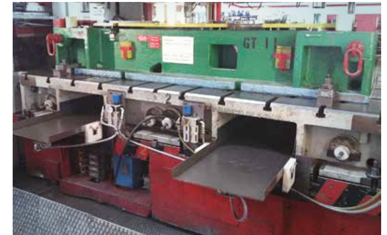
Left: Mounting detail with a PS100 unit with multiple tray design for light parts
