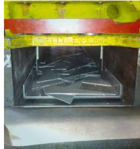
Left: Stamping die with prepared scrap channels for one each PS60 unit with tray
