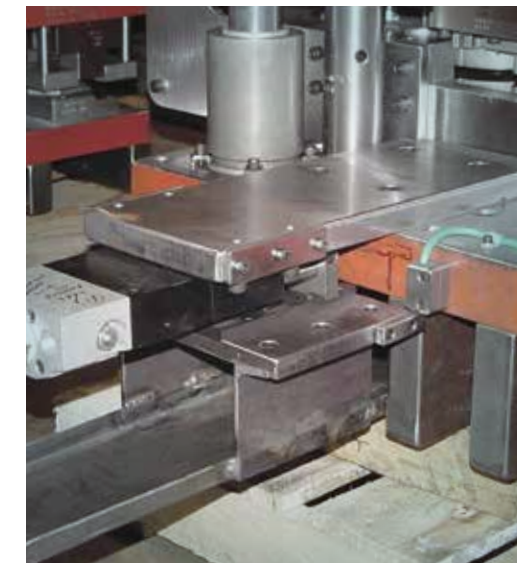
A PS40 mounted directly on the die with removable tray construction and sensory stroke monitoring
