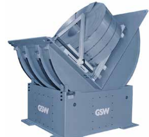
20t upender for up to 2300 mm large coils. Sliding keeper swords for different widths
