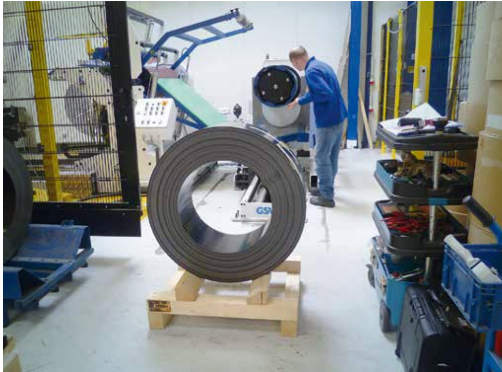
Run-Off. Sheet metal fan Hubert Albrecht is checking the automatic strip clamping function. Besides the new recoiler, the slitting line now has a modern strip brake with semi-automatic processing of the strands, a new line safety and peripheral guarding
